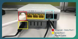
Note: If your ONT was installed before 2020, you will find the ports in the middle, to the right hand side of the box. 4. Ensure the ONT/ Genexis face plate is correctly mounted onto the base unit.
